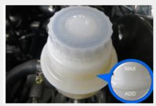
Front engine hood: Marking on brake fluid reservoir
