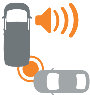
Cross Traffic Alert Helps when reversing out of a parking bay, by warning of traffic approaching from either side. Part of Blind Spot Information System. (Option)
