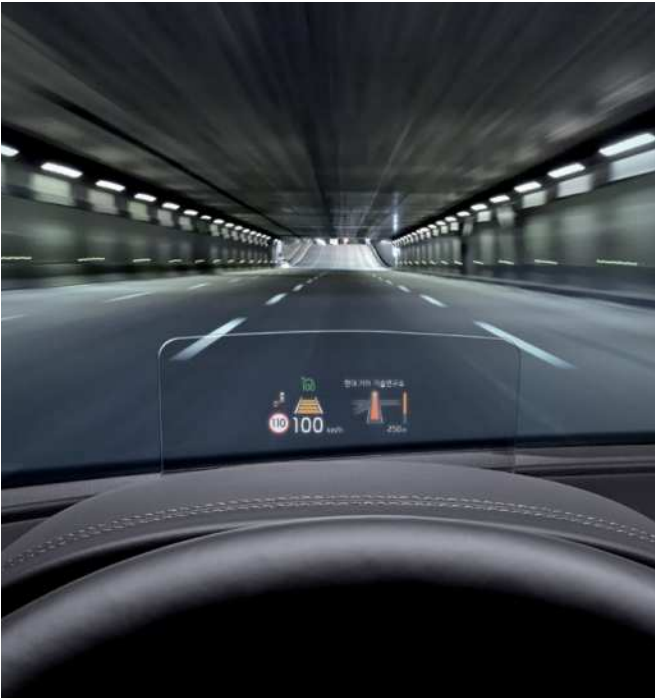
Combiner HUD (Head-Up Display) Diverse driving information is projected onto the windshield to minimize movement of the driver's line of sight and promote safe driving.
