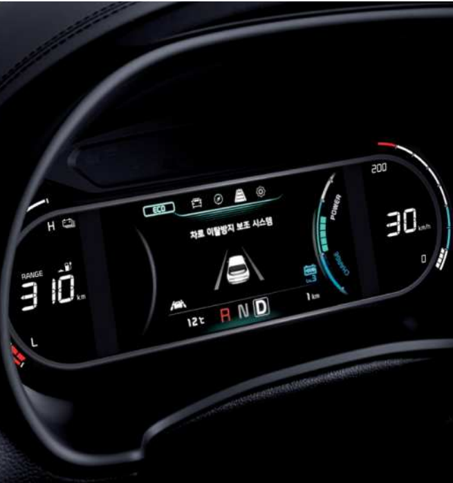
Supervision cluster (7" color TFT LCD) Diverse vehicular and navigational information is displayed through a 7" color TFT LCD monitor with exceptional visibility.
