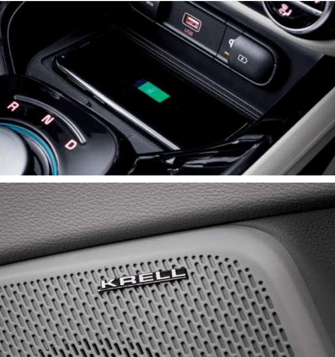
Wireless smartphone charging system Smartphones can be charged without a cable with this high-tech convenience device. ※ A separate charging pad or phone case may be required depending on the smartphone model. May not be compatible with models that do not support the use of adaptors. KRELL premium sound A sound system by KRELL, an American high-end audio brand, renders rich, concert-hall-quality sounds in your car.
